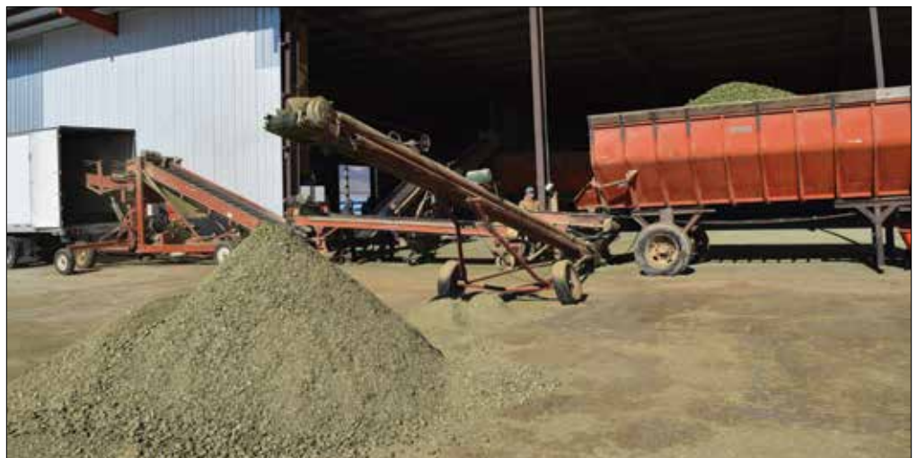
A potato elevator loading a van trailer with the hay remnants piling up to put back through the cuber.
