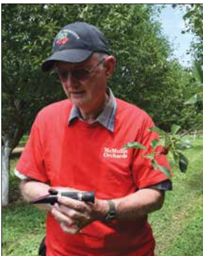
Robert testing the brix (sugar level) in the cherries to determine ripeness.
