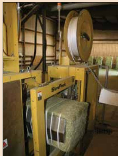
A compressed bale in the compressing machine.
