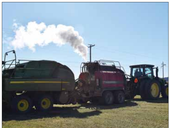
The baling system with the steamer that allows for baling anytime of day.
